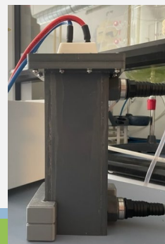
Electrochemical cell prototype Cell configuration: Plate and frame Anode material: BDD Cathode material: Titanium
